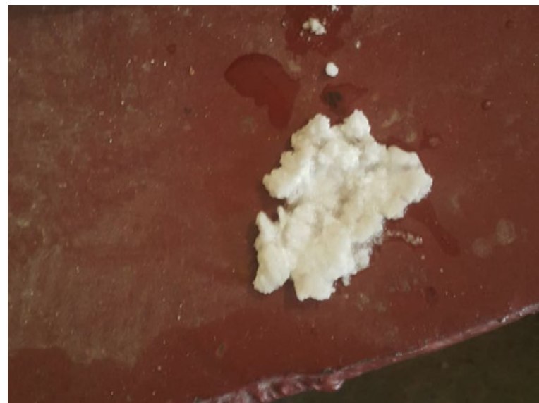
With Vulcan 3000 for 1 month, the scale became soft and easy to remove.
